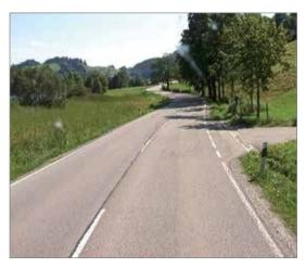
Visibility was improved by removing the obstacle (tree).
