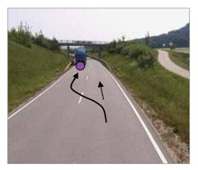
Visibility was insufficient for overtaking due to the slope and the bridge. However, drivers performed overtaking manoeuvres despite insufficient visibility, which caused severe accidents involving longitudinal traffic (rear-end and head-on collisions). Measure
