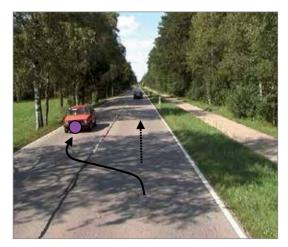
The road provided little opportunities for overtaking while the volume of traffic was quite high. Overtaking despite short time gaps in incoming traffic repeatedly caused severe accidents involving longitudinal traffic (rear-end and head-on collisions). Measure
