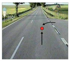
The stop line was no longer clearly visible causing vehicles to turn into the priority road without stopping and colliding with vehicles having the right of way. Measure
