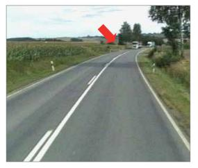
Since the intersection was hard to see, drivers drove too fast in the intersection area which made it difficult for vehicles coming from the minor road to turn into the major road (short time gaps in the main flow).
