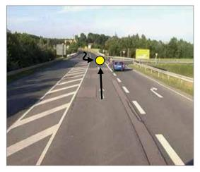
Drivers turning left into the minor road ignored the right of way and collided with oncoming or right-turning traffic.
