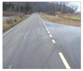
The stop line was renewed to signal drivers turning into the major road in a clearer way that they are obliged to stop.
