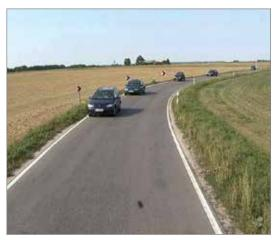
Individually placed bend chevrons and renewed road edge markings indicate the direction of the bend.
