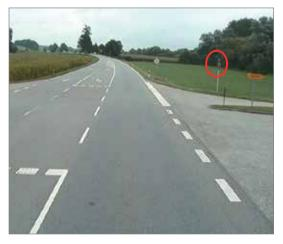
A stop sign indicates the obligation to stop on the minor road and prohibits entering without stopping at the stop line. **BUT:** The entry area is still too wide.
