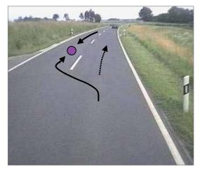
Due to the vegetation at the edge of the road visibility was not sufficient for overtaking, which frequently caused accidents involving longitudinal traffic (rear-end and head-on collisions) during overtaking manoeuvres.
