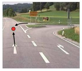
The obligation to stop on the minor road was often ignored with drivers turning into the major road without stopping resulting in a collision with vehicles having the right of way.
