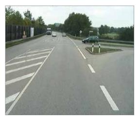
Visibility for traffic turning into the major road was improved by replacing the marker board with posts.
