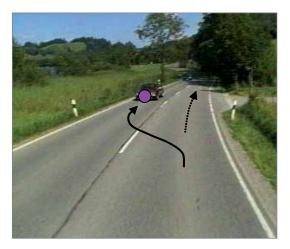
Visibility for overtaking was limited by a tree at the edge of the road. Due to overtaking manoeuvres accidents involving longitudinal traffic (rear-end and head-on collisions) occurred repeatedly.
