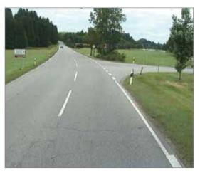
Obstructions reducing visibility for traffic turning into the major road were removed by optimising the installation sites of the signs. BUT: A channelizing island (droplet shape) on the minor road is still lacking. The signposts are not installed according to the regulations.
