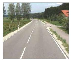
Thanks to the extension work based on the existing structure, the road is safe for traffic again. BUT: The vegetation in the inner bend is still limiting visibility. In addition, the safety distance between the road and the attached bicycle path is insufficient.
