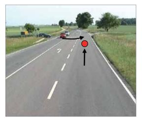
The range of vision of the traffic turning into the major road was very wide inducing drivers to misjudge distances and speeds, not least due to their own high speeds. Turning into the major road without stopping at the stop line led to severe accidents with vehicles having the right of way.
