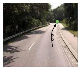
The broken line centre road marking was insufficient to indicate the course of the road and promoted high driving speeds and road departure accidents.
