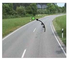
The discontinuity of the road's layout and the poor condition of the road promoted many single-vehicle accidents when the road was wet.
