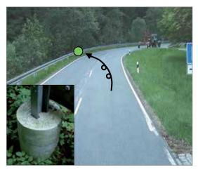
The road's layout was discontinuous and the marking was hard to see. Motorcycle single-vehicle accidents involving a collision with the posts of the steel crash barrier resulted in severe consequences despite the posts' protective casing.
