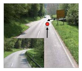
The junction that is located after a bend was not visible from the major road. The destination sign with arrows indicating the directions was installed directly before the intersection and additionally limited the visibility of drivers turning into the major road causing them to collide with vehicles having the right of way.
