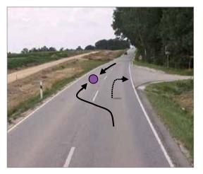
The layout of the road was discontinuous. In addition, this section of the road had numerous access roads and junctions, which promoted risky overtaking manoeuvres of turning vehicles travelling at lower speeds.
