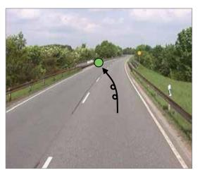
The straight layout of the road incited drivers to drive very fast (speeding). However, visibility was insufficient for overtaking due to the vegetation and the steel crash barrier, which resulted in single-vehicle accidents when overtaking.
