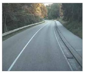
The solid line centre road marking makes the course of the road and the lane limits clearer. In addition, overtaking is banned.
