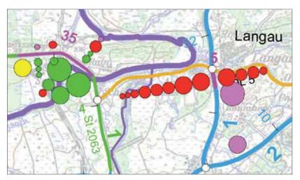
Figure 1: Detail of a three-year accident type map with accident blackspots (magentacoloured line) 2000-2002 for federal and state rural roads in Bavaria
