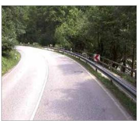
Individually placed bend chevrons indicate the direction of the bend. When a vehicle departs from the road, steel crash barriers prevent it from colliding with a tree which might have severe consequences.
