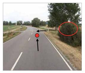
The visibility splay (range of vision required for a driver to safely turn into a major road from a stop) at the intersection was insufficient. Accidents with vehicles having the right of way occurred as vehicles turned into the major road despite of bad visibility.
