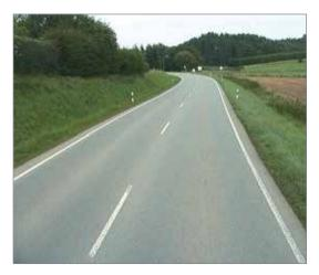
The flatter slope improves visibility and makes it therefore easier for the drivers in the main flow to see the course of the road, including the intersection.
