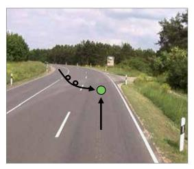
The single solid line centre road marking was insufficient to indicate the course and threelane, single-carriageway layout of the road, which promoted single-vehicle accidents. Measure
