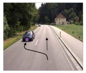
Visibility was not sufficient for overtaking. Due to overtaking manoeuvres performed despite insufficient visibility, accidents involving longitudinal traffic (rear-end and head-on collisions) occurred repeatedly.
