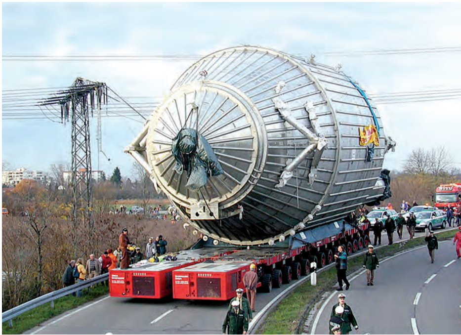
Fig. 2: Large-volume and heavy-duty transport
