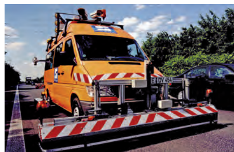
Figure 1: Vehicle for measuring longitudinal and transverse unevenness and substance characteristics
