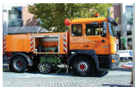
Figure 2: Vehicle for measuring road grip
